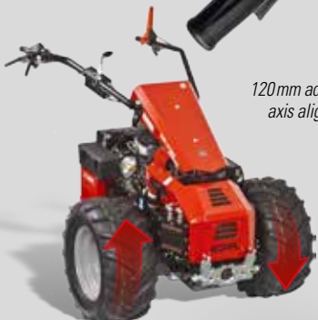
Turn-around-active-steering Maximum comfort and ground protection.
