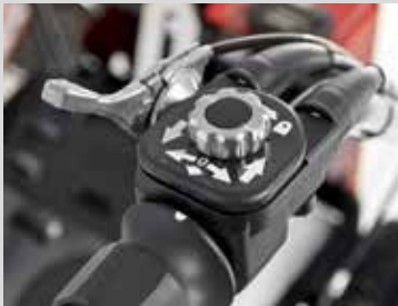
PTO independent speed adjustment
