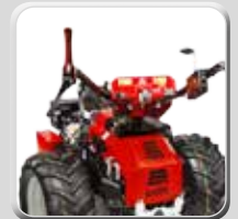
Rear view: Hydro Athlet-handlebar 180° rotatable with 20° lateral offset
