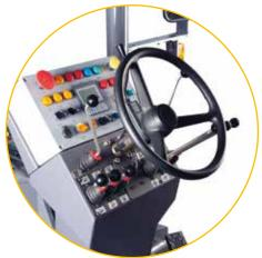
Open canopy – FOPS-approved, electrical equipment with protection class IP65
