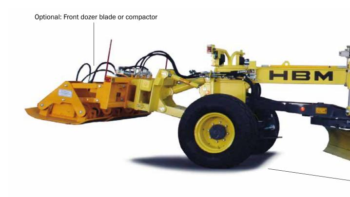
The BG 110-M was developed in collaboration with mining specialists especially for use in mining applications. With a height of only 1.80 m and an overall length without attachments of less than 7.40 m, it can be operated in even the smallest of mines in the world.
